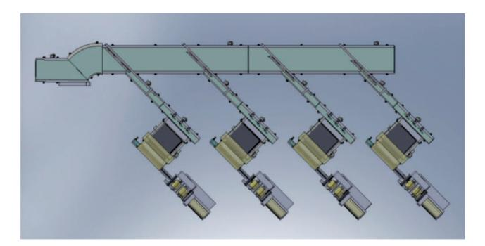
Wrapping line for products in random This wrapping system includes Automatic product dividing system Multi rows feeding system Servo wrapping machine
