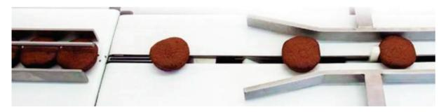
From simple mechanical direct feeding device, to quantitative feeding system which measure length or quantity, product group, all electronic, has push rod. These system can separate or measure product, is special customized solutions which in order to effectively packaged the biscuits into pile or into strips.
